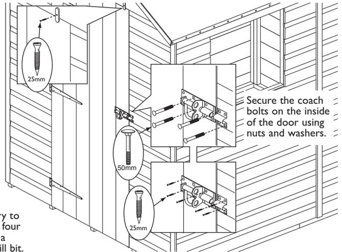
Secure the coach bolts on the inside of the door using nuts and washers.
