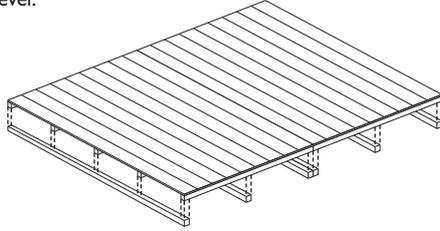
To "VALIDATE" the guarantee, this item should be erected on 50mm x 50mm treated wooden or similar bearers (**These are not supplied with the kit.**) Ground contact must be avoided.
