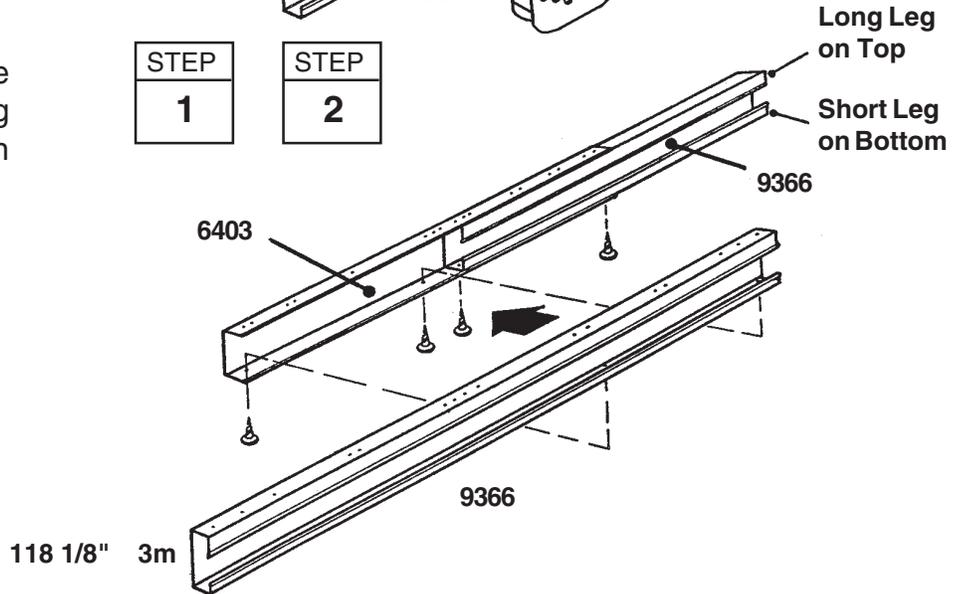
**3** Position **door slides** onto the legs, from the end of door track assembly, as shown in the end view.
