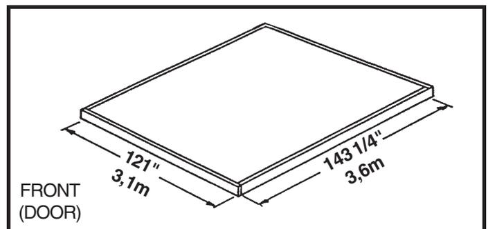
Note: Finished Slab dimensions, with lumber removed.
