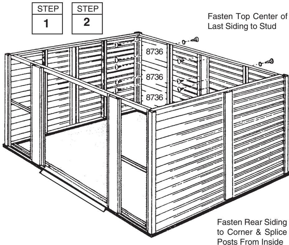
**3** Slide **front siding** into channels of corner post and door jamb. This siding is fastened from the inside, using screws into post and jamb.
