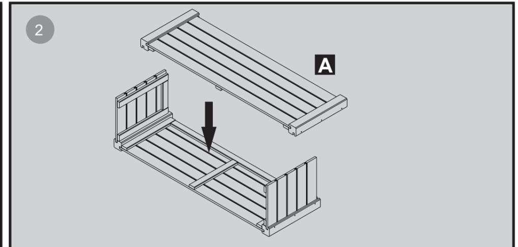
Place both sides together and position so that all sides are flush and secure.
