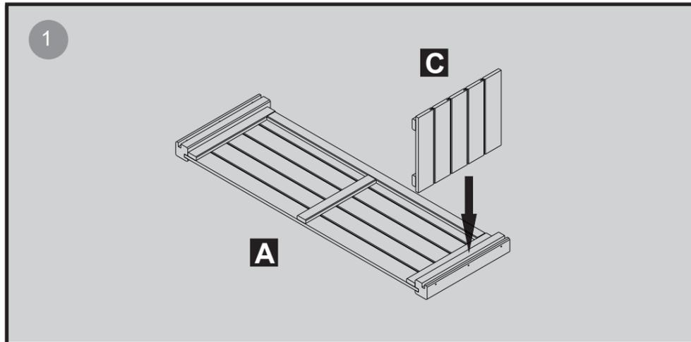
Place the small insert into the side as shown.
