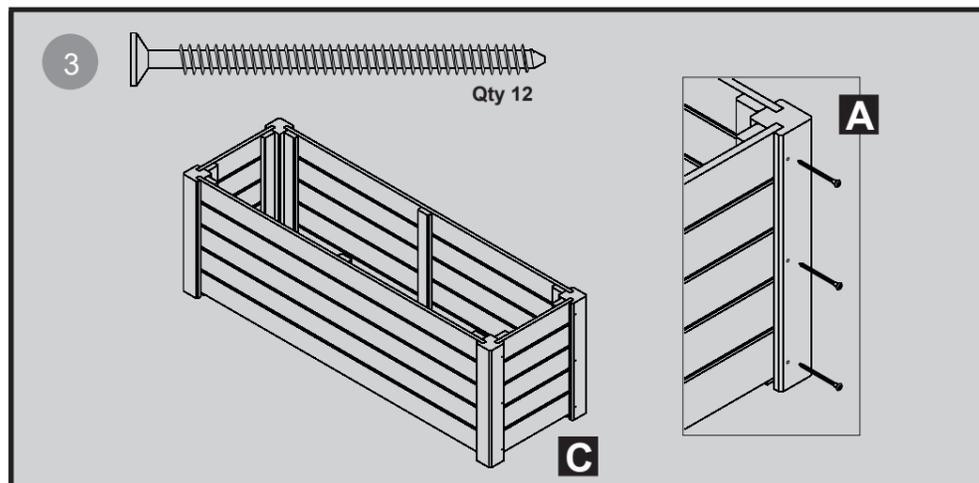
Pre drill holes as shown on the side. Secure the sides to the small inserts.
