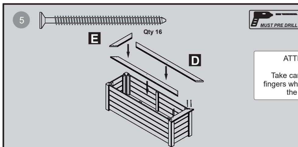
Position the wooden cills before fixing and take time to make sure that these line up correctly and are square. There should be an overhang of approximately 20mm from the posts. Once in place pre drill the holes as shown and fix.
