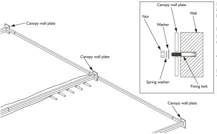
Put the canopy frame into position, ensure the feet are flat on the floor and the tracks are level using a sprit level. Mark the wall with the position of the 4 holes of each wall plate.
