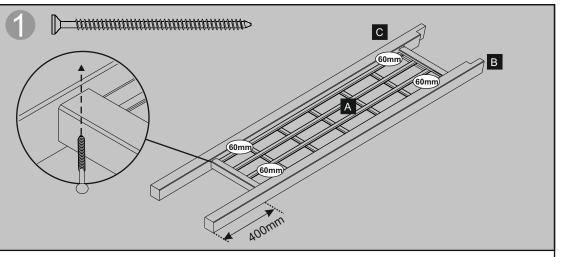
Lay 1  $\times$  B and 1  $\times$  C posts on the ground with both notches facing inwards. Position the trellis 400mm up from bottom of the posts (the flat ends). Secure the trellis to the posts using 4  $\times$  60mm screws through the top and bottom of the framework. Repeat procedure to connect remaining trellis and posts.
