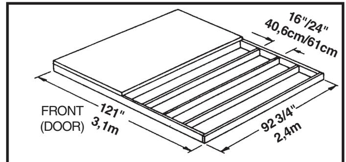
**Note: Platform/Slab will extend 9/16" (1,4cm) beyond floor frame on all four sides. Seal this 9/16" of wood with a roofing cement (not included), or bevel this 9/16" of concrete when pouring, for good water drainage.**
