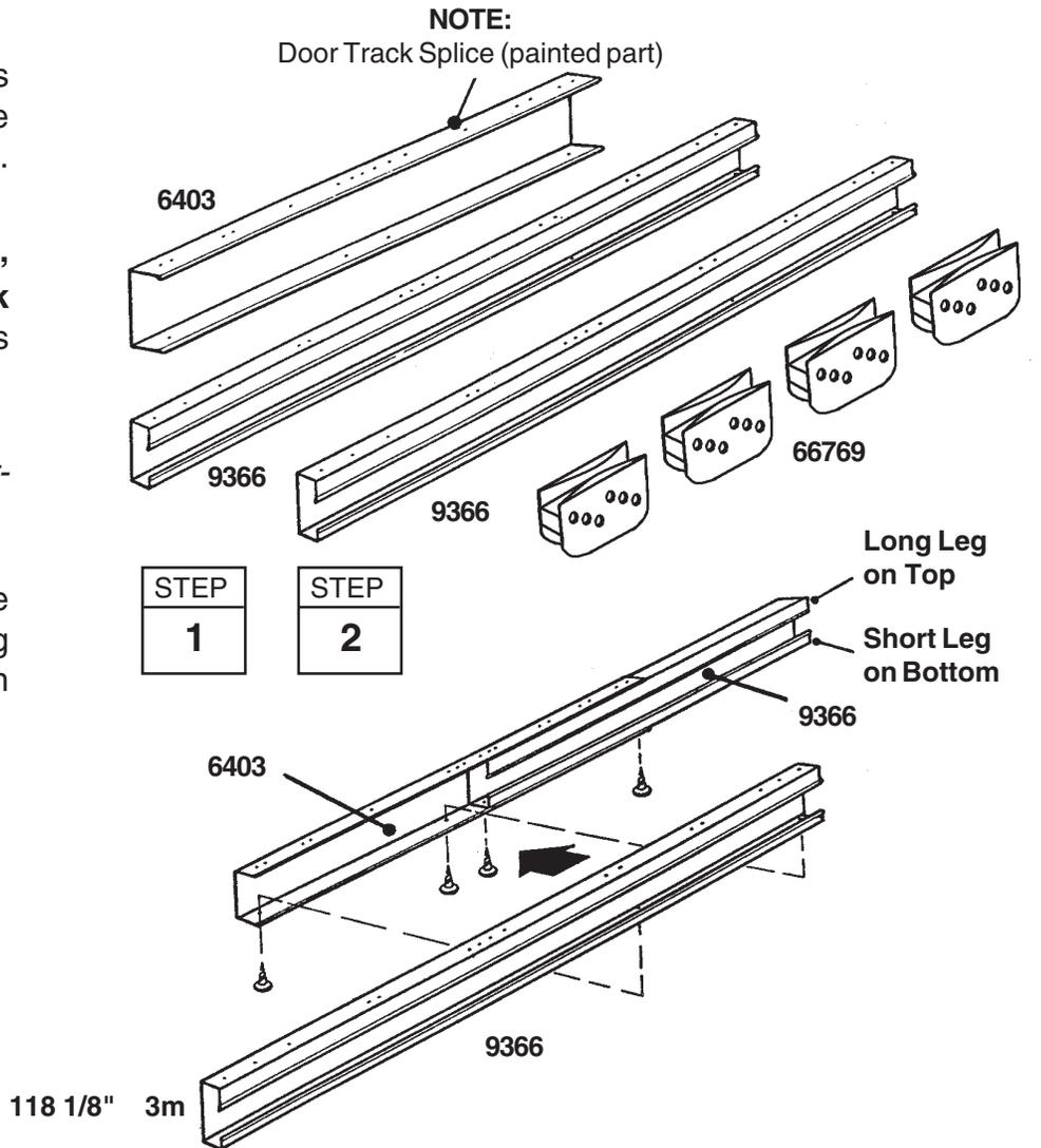
**3** Position **door slides** onto the legs, from the end of door track assembly, as shown in the end view.
