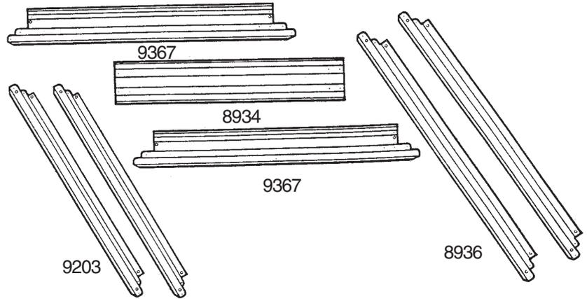
**1** Place the **front floor frames** as shown. Center the **ramp**, with drain holes facing outside, on top of the two front floor frames. Join the frames by inserting eight screws.
