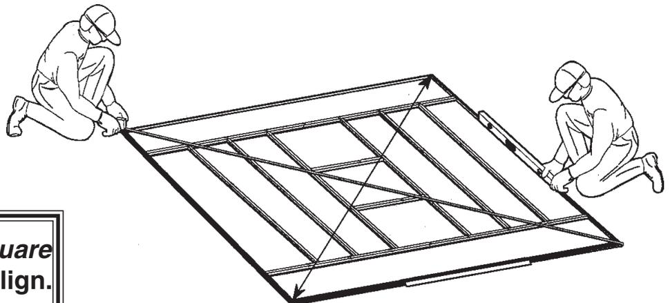
**The floor frame *must be square and level* or holes will not align.**
