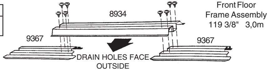
**2** Overlap the **side floor frames** and the **rear floor frames** as shown. The holes in these pieces will align when the pieces are positioned with correct amount of overlap. See the illustrations below for the proper overall length of the side and rear floor frames. Join the frames by inserting four/five bolts into each frame set as shown.
