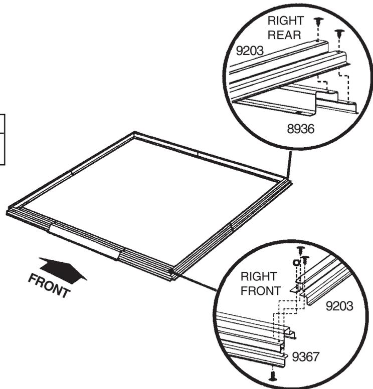
**2** Measure the floor frame diagonally. When the diagonal measurements are equal, the floor frame is square.
