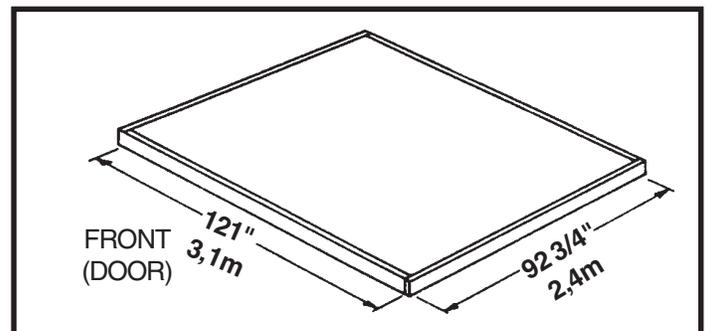
**Note: Finished Slab dimensions, with lumber removed.**
