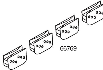
**1** Position **door slides** onto the legs, from the end of door track, as shown in the end view.
