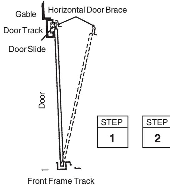
**1** From inside the building, put the bottom of the right door assembly (on your left when you are inside the building) behind door jamb into the front frame track.
