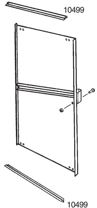
**5** Attach the **lower door guides and bolts** as shown.
