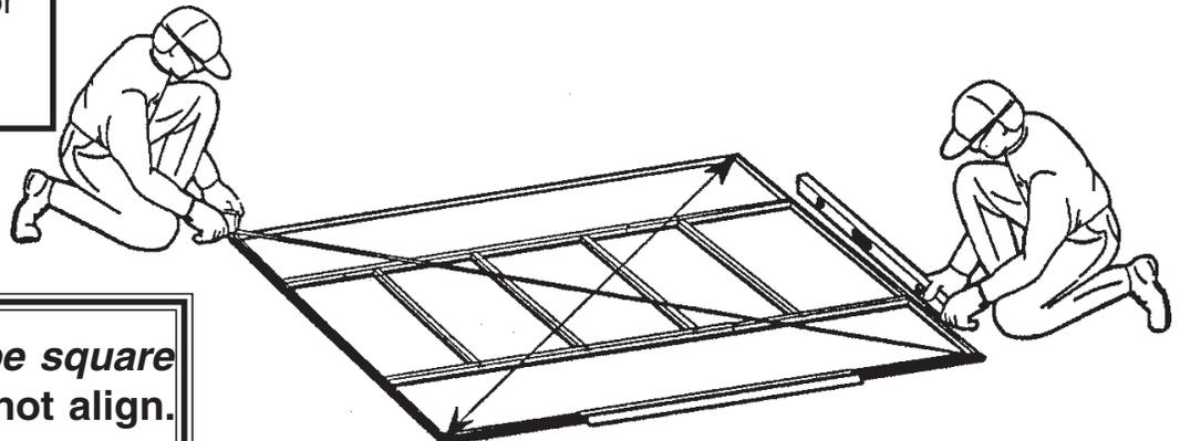
**The floor frame *must be square and level* or holes will not align.**
