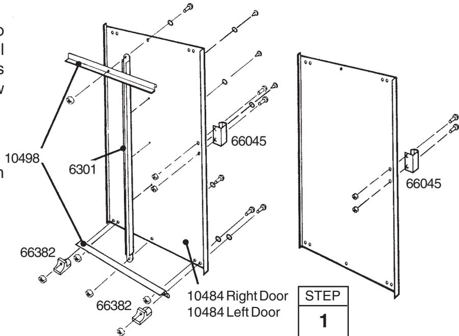
**2** Hold the **vertical door brace** against the center of the inside surface of the door and turn the screw to hold the vertical door brace in place. Fasten to door above and below center connection using 2 screws.
