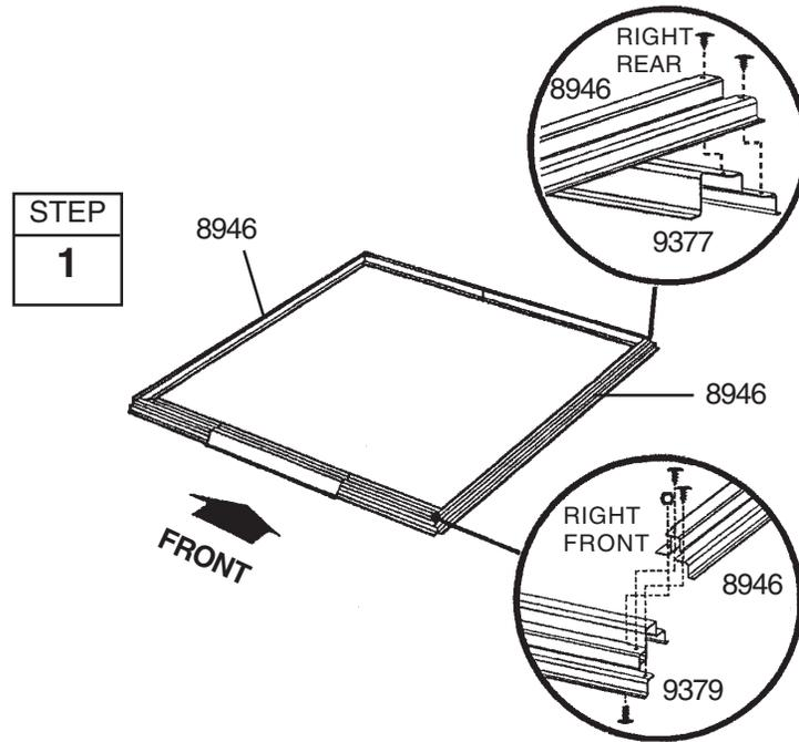
**When Diagonal Measurements are Equal the Floor Frame is Square.**
