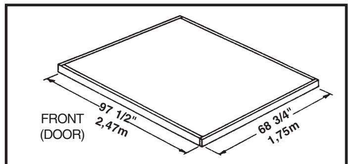
Note: Finished Slab dimensions, with lumber removed.
