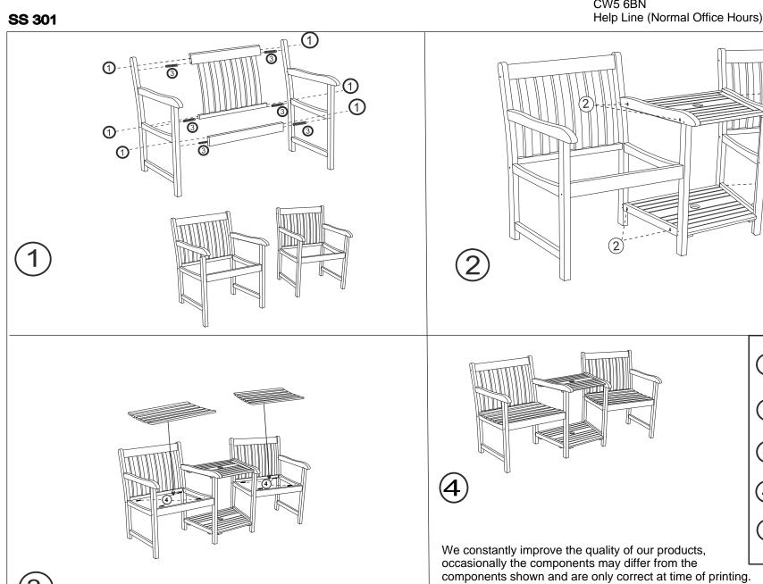
(1)Screw 7x90=12pcs Screw 7x50= **8**:pcs (3)Wood 10x30=12pcs Screw 4x40 x 8 (5) allen key x 1 pc
