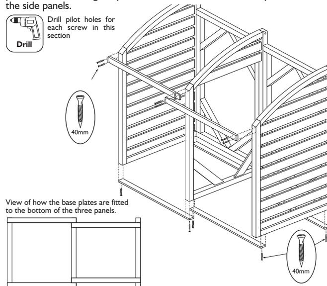
View of how the base plates are fitted to the bottom of the three panels.
